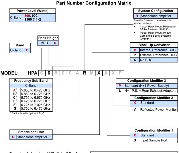
**Example** - A standalone 800W GaAs C-Band 6RU Rack Mount SSPA with standard N+1 external power supply and an optional internal reference block up converter is part number: **HPAC6800ARMXXXP**.
